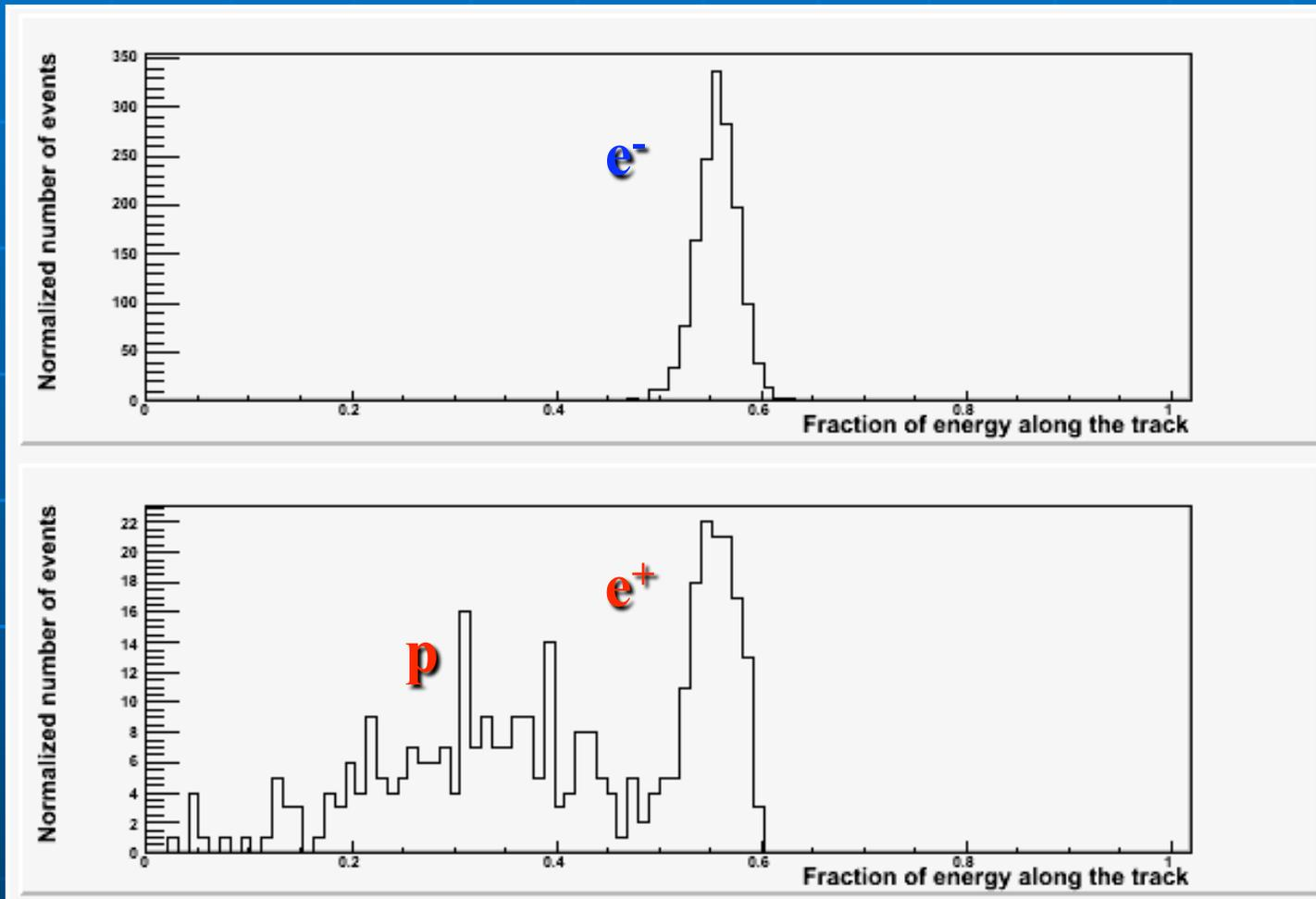
Fraction of charge released along the calorimeter track (left, hit, right)
