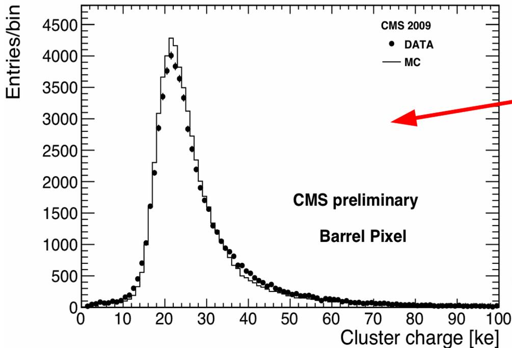
Charge corrected for track incident angle
