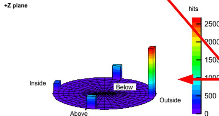
Increased response in one of the sensors compared to others indicates movement of beam towards this sensor
