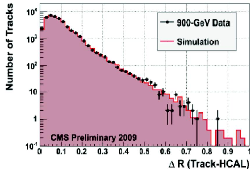
Agreement with simulation validates track cluster link efficiency, alignment between tracker and calorimeters and energy sharing between ECAL and HCAL
