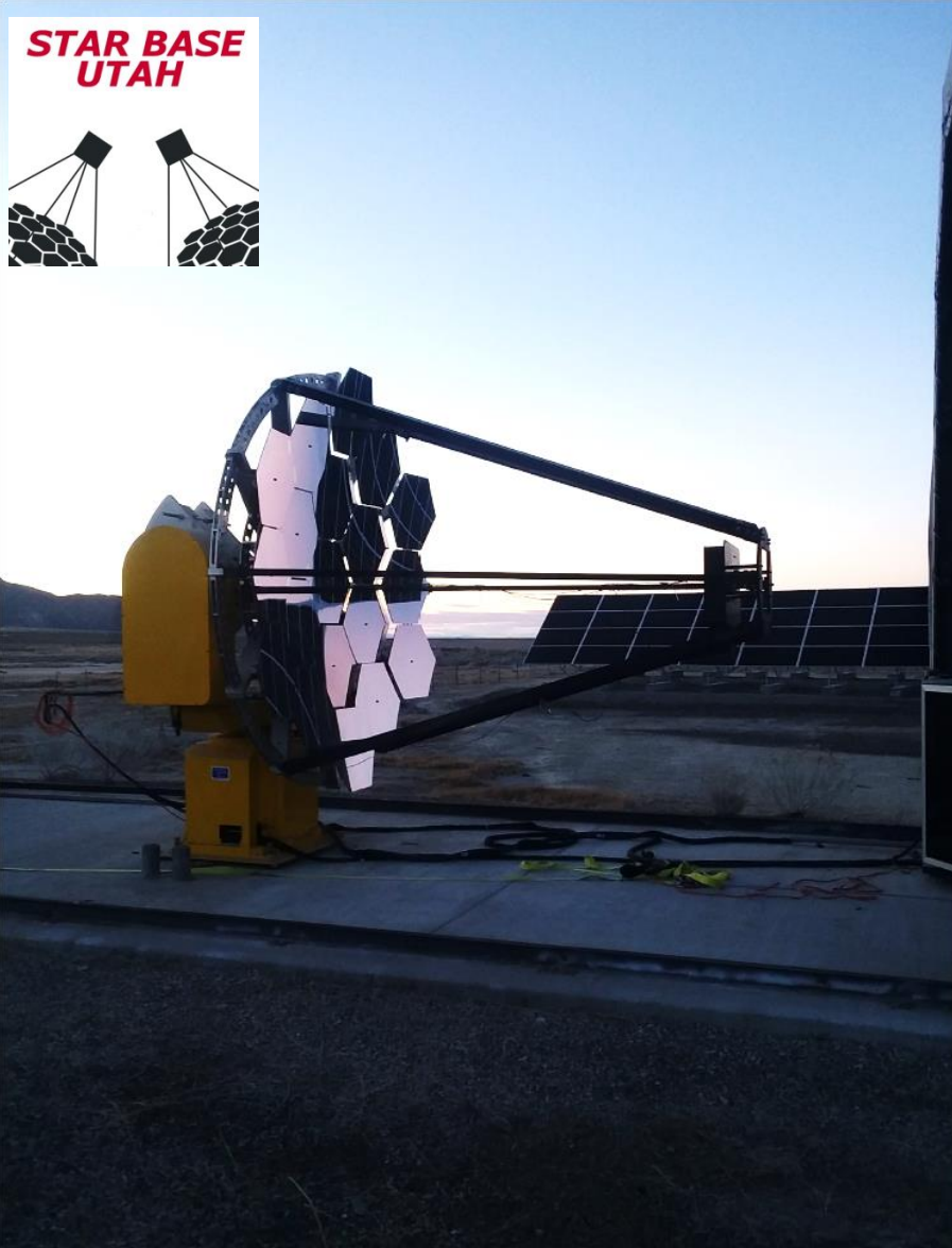
Left: One of the StarBase telescopes, having 19 hexagonal mirror facets with total diameter of 3 m. Right: Light is detected by the intensity interferometry camera consisting of a single PMT 'pixel'
