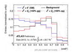
Background  $|\cos\theta^*|$  shape interpolated from  $m_{\gamma\gamma}$  sidebands into signal region (122 to 130 GeV)
