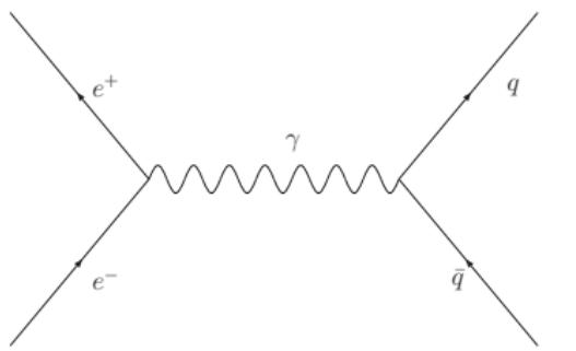
Born diagram for  $e^+e^- \rightarrow \gamma \rightarrow q\bar{q}$
