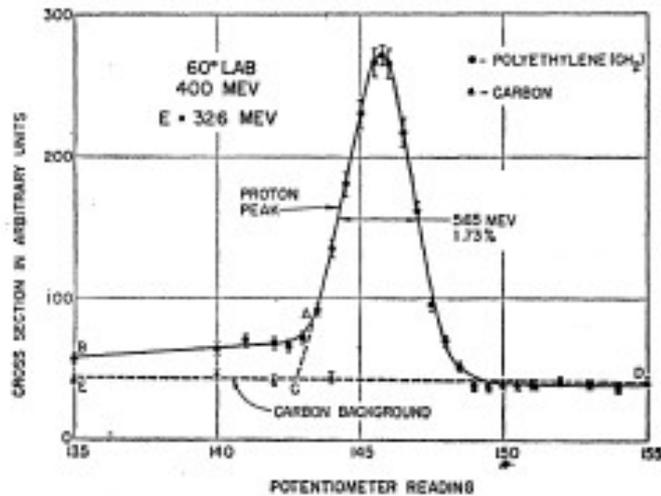
FIG. 25. Elastic scattering of 400-Mev electrons from protons in polyethylene at a laboratory angle of 60°.
