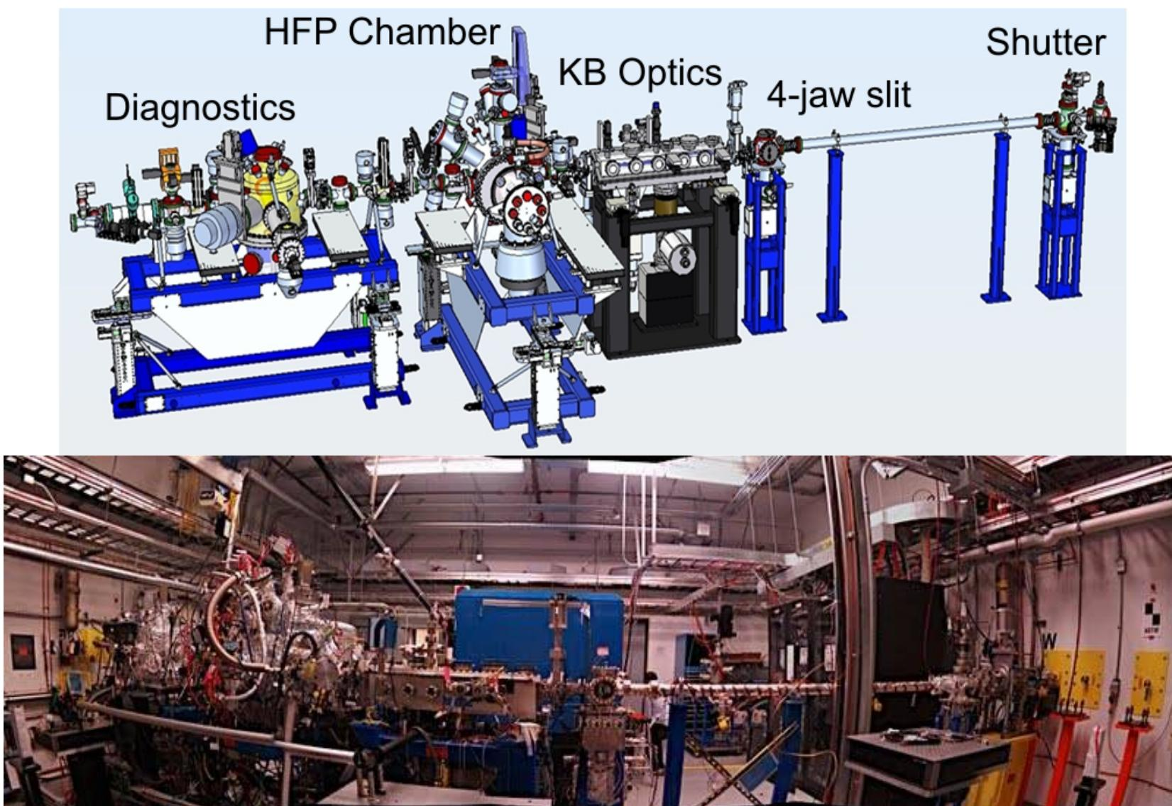
The AMO instrument is 4 distinct vacuum chambers with different functions
