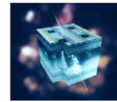
Illustration of microelectronics circuitry integrated with a sensing medium as a single monolithic active detector. (© ECFA collaboration)
