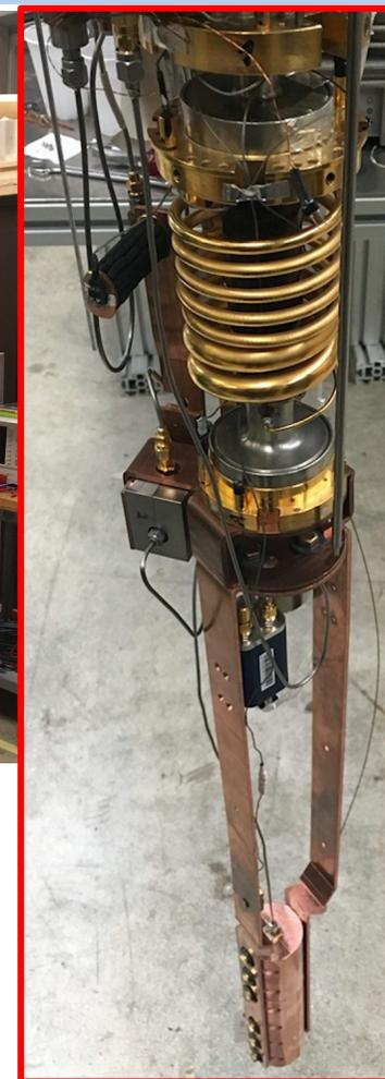
Dilution insert with rf electronics and cavity
