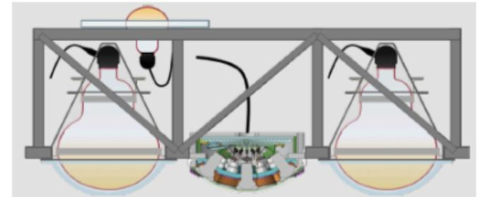
*Potential combination of 50cm PMTs and multi-PMT modules*
