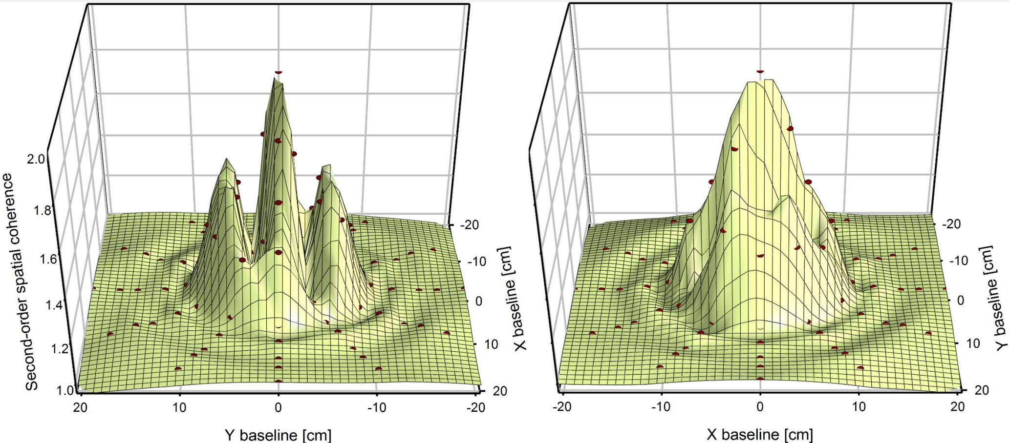
Second-order coherence  $g(2)$  for an artificial binary star with each component of diameter  $\sim 1$  arcsec.
