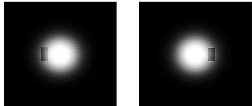
Gaussian source with rectangle, reconstructed by Gerchberg-Saxton algorithm
