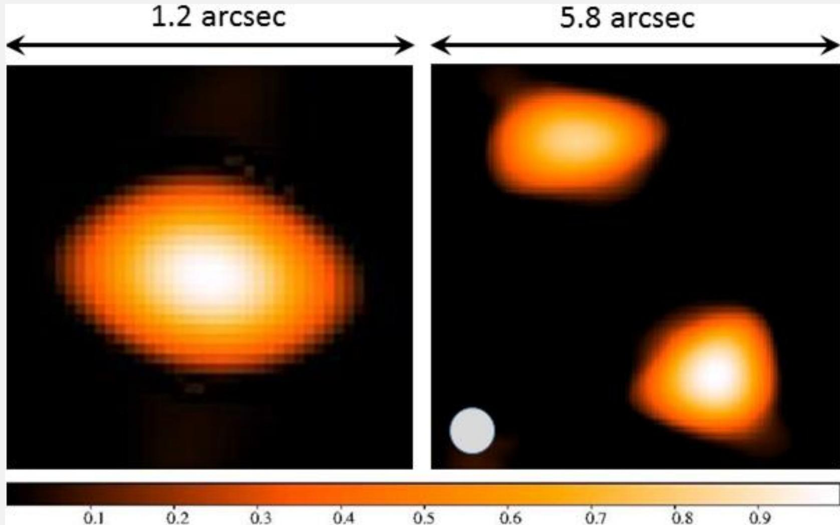
Optical images reconstructed from intensity interferometry.
