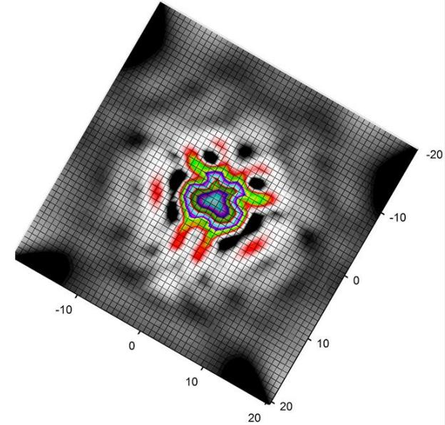
Measured second-order spatial coherence  $g^{(2)}$  from intensity interferometry over 180 telescopic baselines. The source is an artificial binary star with differently large components. The structure corresponds to the pattern that would be produced by coherent light undergoing diffraction in a corresponding aperture.
