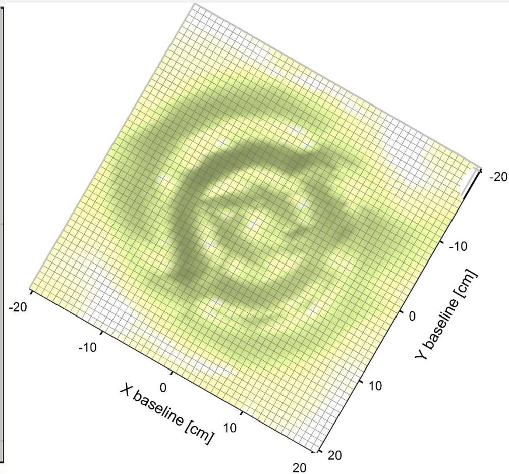
Intensity interferometry measurements with 100 different telescopic baselines. The data largely fill the interferometric  $(u,v)$ -plane of the second-order coherence  $g(2)$  for an artificial star, somewhat irregular and elliptic, with angular extent just below 1 arcsecond. At right, the projection of the 3-D mesh is oriented straight down, showing [the modulus of] the source's Fourier transform ('diffraction pattern').
