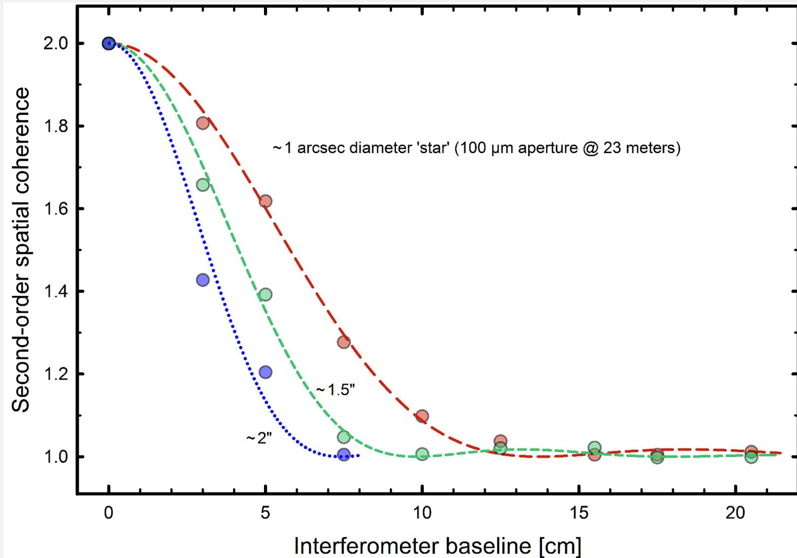
Second-order coherence  $g(2)$  measured for artificial single stars of different angular sizes. Superposed are Airy functions for circular apertures (squared moduli of the Fourier transforms).
