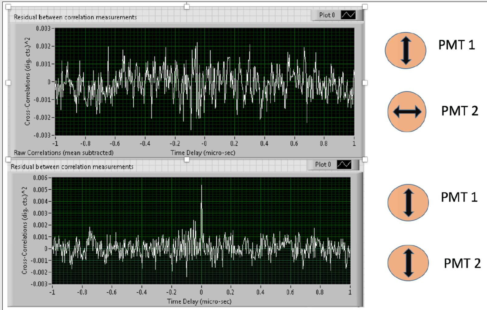
**Temporal coherence from a Hg arc lamp in the laboratory at the University of Utah. Upper plot: Non-correlation with perpendicular polarizations. Lower: Observed 2-photon correlation with parallel polarizer configuration.**
