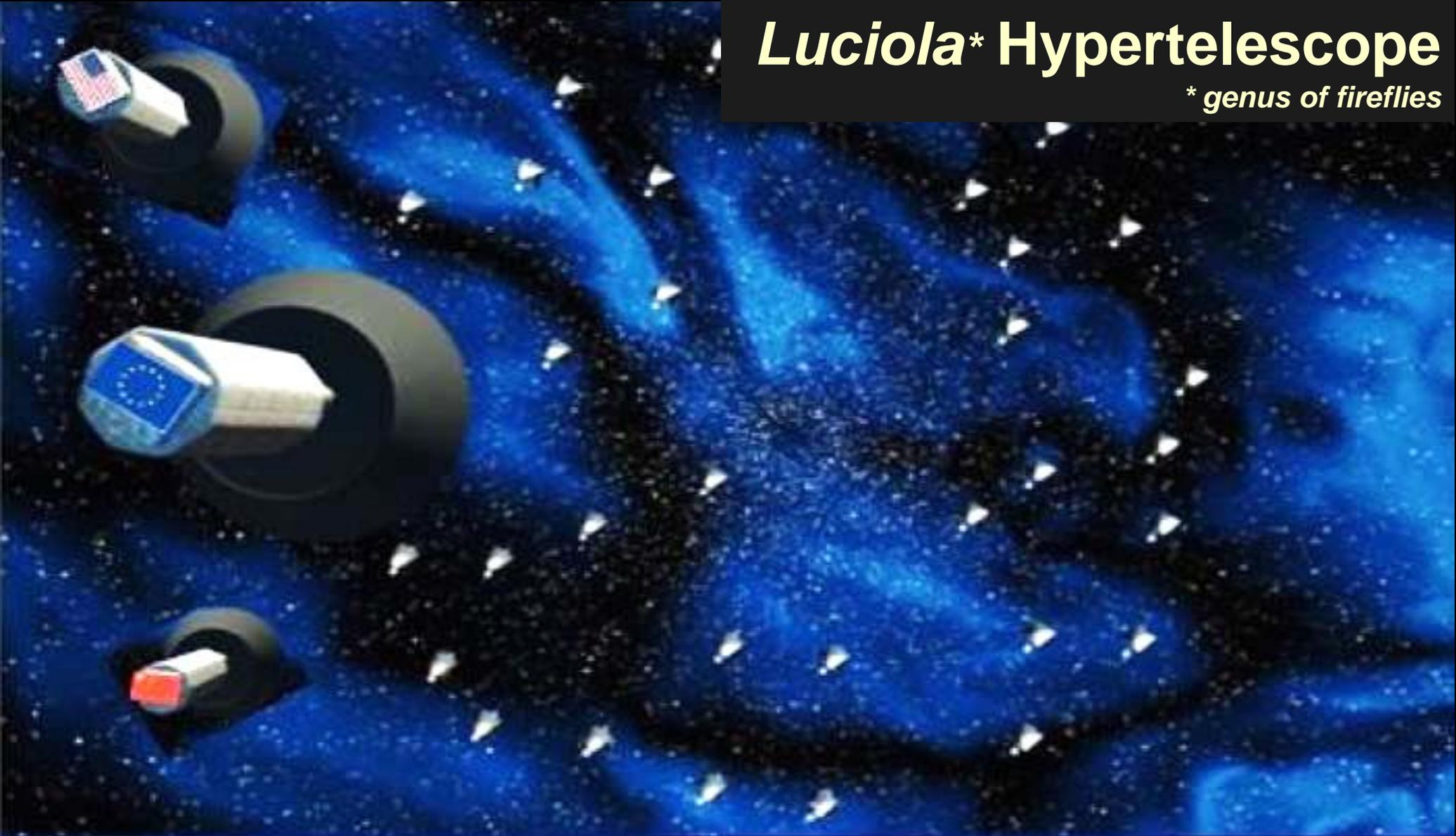
The *Luciola* flotilla of many small collector mirrors operates like one giant diluted mirror. Focal beam-combiners independently exploit the sky image formed at the focal surface.
