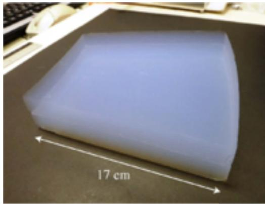
Silica Aerogel cut by water-jet
