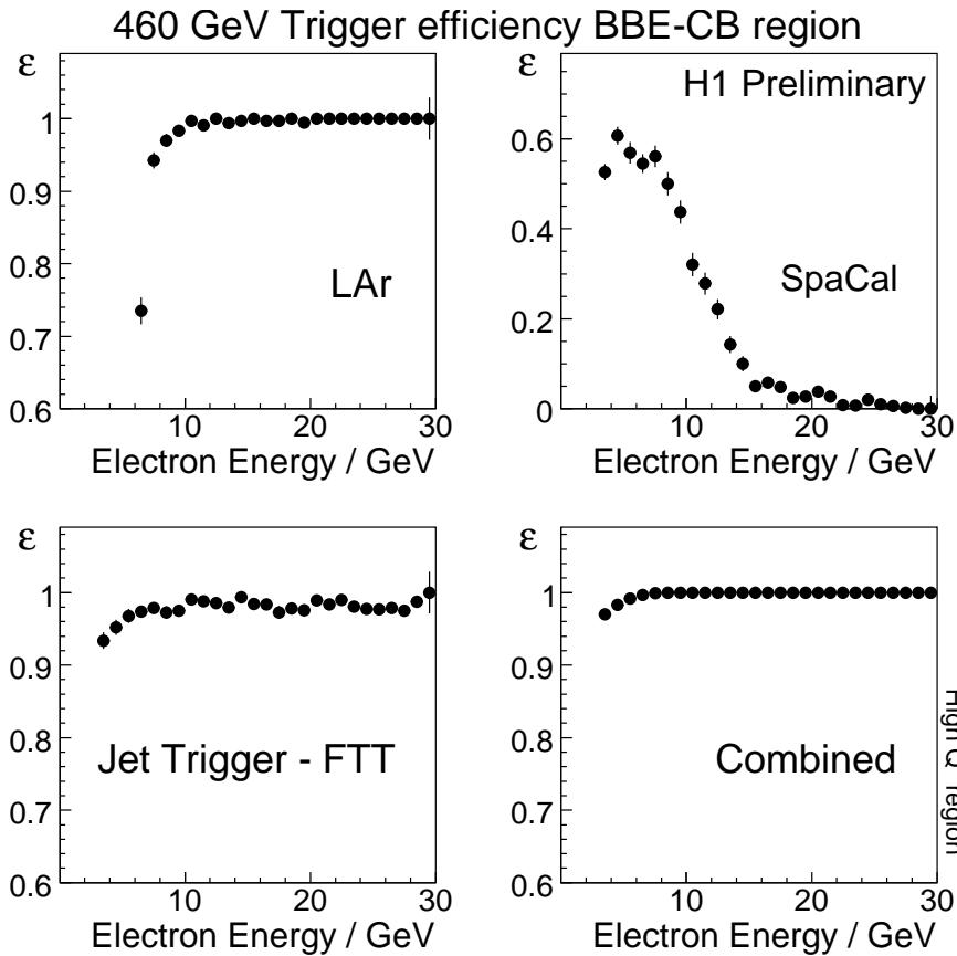
Jet (real time clustering) - FTT (fast track) trigger requires cluster-track match at high level trigger. Jet trigger fully commissioned in 2007.
