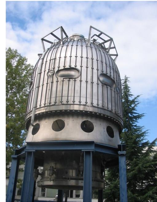
A bubble chamber is a vessel filled with a gas in a phase of superheating. The passage of charged particles ionizes the gas and bubbles are formed along the path
