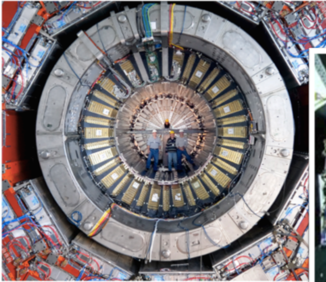
CMS calorimeter system at LHC (CERN) (the humans are not part of the experiment)
