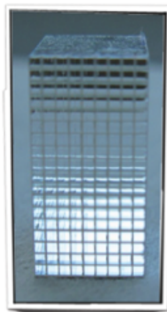
LYSO matrix [Proteus] 9x18 crystals; each: 0.71x0.71x15 mm 3
